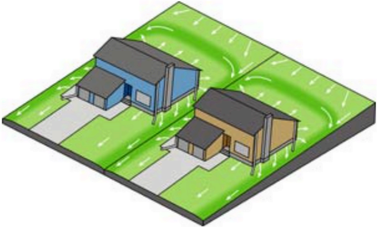
Above: A schematic of back to front grading (City of Winnipeg, n.d.).
