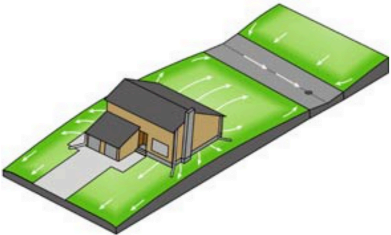
Above: A schematic of split side grading (City of Winnipeg, n.d.).
